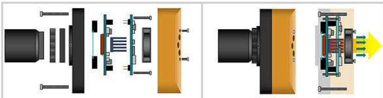
The **Opticstar PX-137C CoolAir** (colour) and **Opticstar PX-137M CoolAir** (monochrome) cameras incorporate the latest scientific CMOS technology. The Sony IMX035 sCMOS, 1/3" sized sensor (diagonal) offers the ideal combination of high definition (1.3 megapixels), high sensitivity and high speed. The **PX-308C CoolAir** (colour) is the 3 megapixel CMOS version.
