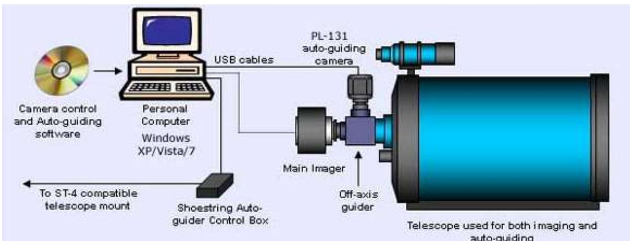
It is recommended that for single telescope setups, the telescope should be 200mm in aperture or greater, since the light will be split by the off-axis guider accessory. In a dual telescope system a smaller dedicated guide scope can be used as shown below. It is recommended that the aperture of the dedicated guide scope should be 80mm or greater.
