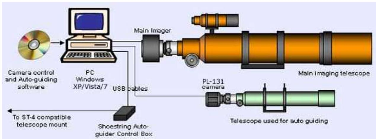
Auto-guiding is a cost effective technique to greatly improve the tracking accuracy of a motorized GOTO mount when long exposures are required for deep sky imaging.
