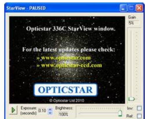
On the main panel, the exposure time can be entered in seconds and milliseconds. Longer exposure times increase light gathering and sensitivity but reduce the camera's frame rate. The **Gain** value can be used to increase the sensitivity of the camera by up to 100%. This signal amplification takes place in the camera and it is combined with noise reduction electronics.
