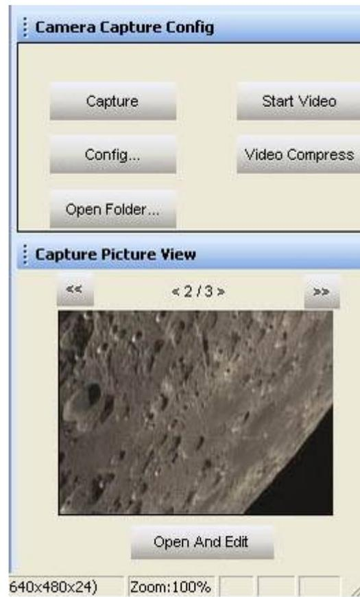
The location of the stored file(s) can be specified by clicking the **Config** button. By default, video data is stored uncompressed in order to preserve high image quality. Optionally, it is possible to compress the AVI files by clicking the **Video Compress** button.
