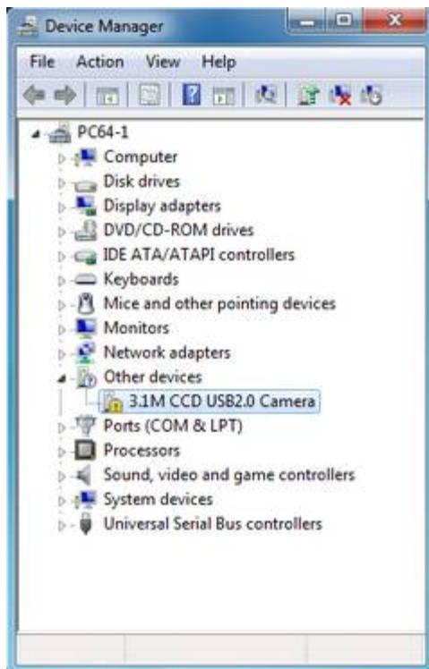
Once connected to the computer, the **Device Manager** will show the camera.
