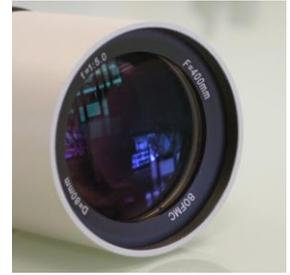
Be careful and always make certain that the nozzle is propellant free. Hold the compressed air-can the right way up as otherwise they can discharge liquid propellant which will stain the optics. Stains on optics can be removed with optical cleaners used to clean photographic lenses. Always use compressed air at very low pressure as contaminants that may have landed on the lens could scratch the glass surface, never rush the cleaning process.
