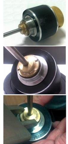
Notice the two grooves on the brass part of the rotational mechanism.
