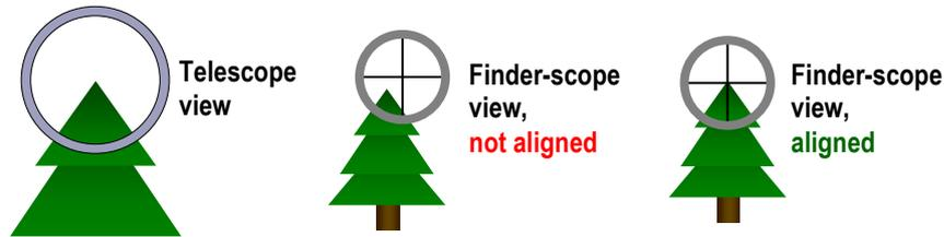
The finder-scope is now aligned to the main telescope. You can check and refine alignment on a night sky object like a star if required. Please note that the view will not be the right way up and views will differ depending whether a diagonal is used or not. If you do not use a diagonal you will need an extension tube to reach focus.
