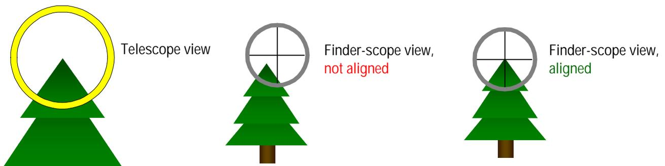
The finder-scope is now aligned to the main telescope. You can check and refine alignment on a night sky object like a star if required. Please note that the view will not be the right way up and views will differ depending whether a diagonal is used or not. If you do not use a diagonal you may need an extension tube to reach focus.
