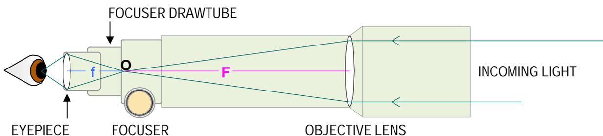
Magnification depends on two factors. The focal length of the telescope and the focal length of the eyepiece used. To calculate the magnifying power an eyepiece gives, simply divide the focal length of the eyepiece into the focal length of the telescope.
