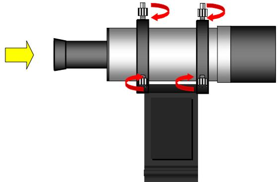
Once Mount the assembled finder-scope to the telescope and secure it in place. Attach the telescope to a mount/tripod.
